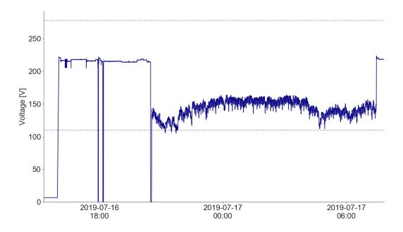
Figure 38: Variable mostly stabilizable undervoltage, then return to usable range, device N-001.
