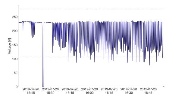
Figure 40: Rapid fluctuations, device N-054.
