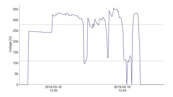
*Figure 42: Undervoltage to overvoltage several times within a 15-minute span, device N-082.*
