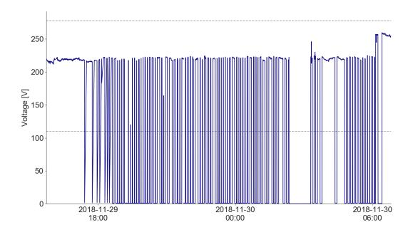
Figure 30: Multiple interruptions, device K-198.
