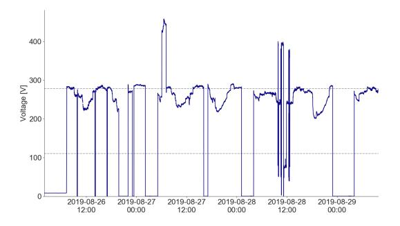
*Figure 45: Fifty (50) minutes of overvoltage reaching 456 V, and another overvoltage the next day. This is device N-067, the same one in Figure 31, and shows a similar pattern of daily variation.*
