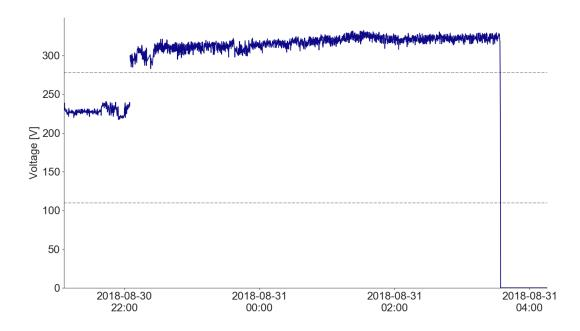
Figure 43: Overvoltage, device N-006.
