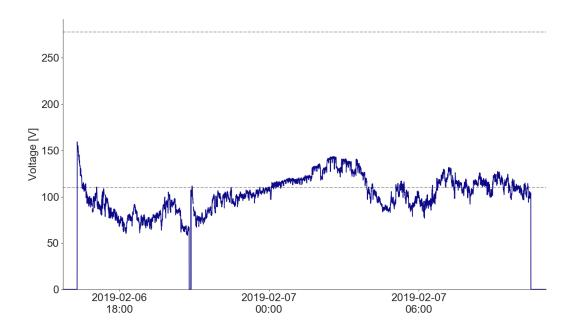
Figure 32: Voltage varying near the border between stabilizable and unusable over 12 hours, device N-044.
