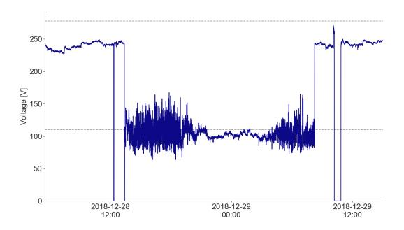
Figure 33: Voltage varying near the border between stabilizable and unusable over 19 hours, device K-001.
