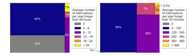
Figure 12: Percentage of devices that reported interruptions longer than 48 hours (left) and longer than 30 minutes (right) in Kenya.
