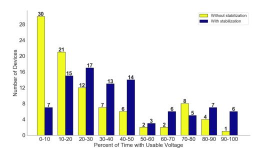
Figure 9: Number of devices in Nigeria by percentage time of usable voltage, showing the impact of stabilization.
