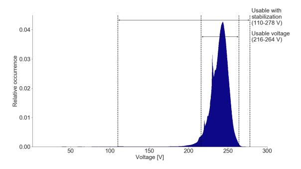
*Figure 15: Line voltages reported by devices in Kenyan facilities during the study period (normalized to 1). Mean is 238.3 V; standard deviation is 16.0 V.*
