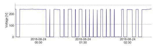
*Figure 14: Time series plot of voltage reported by a device in a Kenyan facility. The voltage range usable with stabilization is between the horizontal dashed lines. Device K-026.*
