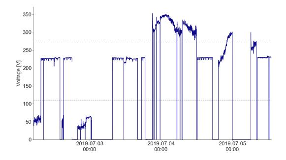
Figure 41: Usable voltage, overvoltage, undervoltage, and zero voltage over a 3-day period, device N-044.
