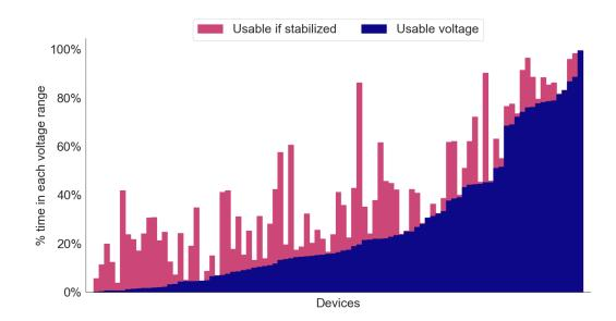
Figure 48: Percentage time in each voltage range for all 93 devices in Nigeria.
