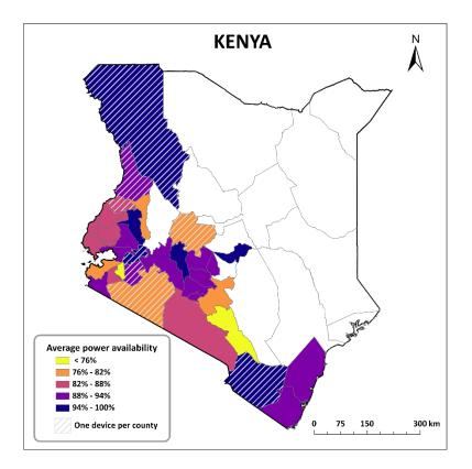
*Figure 26: Average availability of usable voltage by county, as reported by devices in Kenya during the study period (not measured in counties with no color coding). Cross hatching denotes counties with a single device.*
