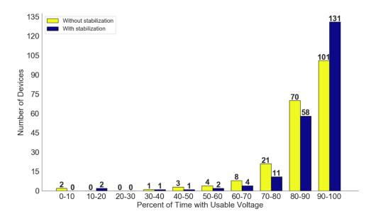
Figure 8: Number of devices in Kenya by percentage time of usable voltage, showing the impact of stabilization.
