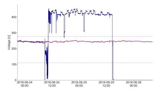
Figure 17: Voltage as a function of time during the study period for two devices in Kenya, contrasting usable voltage with a day-long overvoltage. The voltage range usable with stabilization is between the horizontal dashed lines. Blue trace is device K-117; the purple trace was from a device not in the study.
