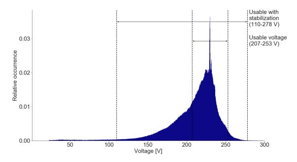
Figure 16: Line voltages reported by devices in Nigerian facilities during the study period (normalized to 1). Each x-axis bin represents 0.1 V. Mean is 209.9 V; standard deviation is 33.5 V.
