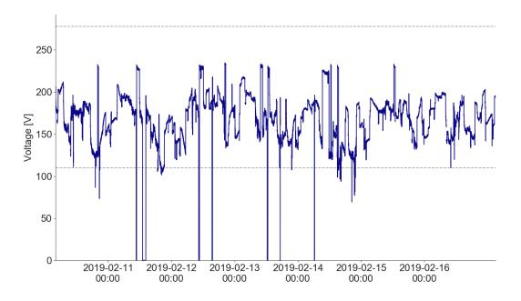
Figure 34: Variable voltage mostly in the stabilizable range over a week, device N-049.
